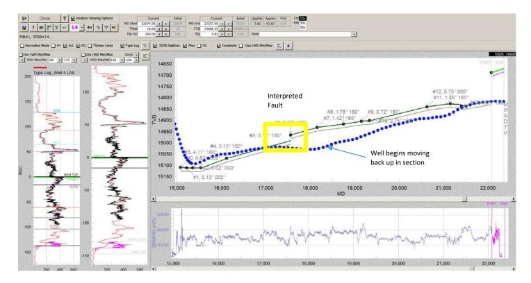
Notice that the well passes through the "payzone" bed multiple times. You can expect to frequently encounter the same LWD signatures as the well moves laterally, which requires stretching, shrinking, and reversing the direction of the log curve on the interpretation track. The well may also encounter faults, in which case you will have to adjust the depth of a strat block by detaching it from the previous strat block.
